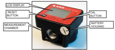
The measurement electronics and the LCD display are fitted in the top part of the meter, isolated from the fluid-bath measurement chamber and sealed from the outside by means of a cover
