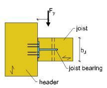
Figure B.3. Joist bearings fastened with nails and dowels for loading HORIZONTAL
