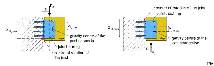
ure B.2. Joist bearings fastened with bolts or metal anchors and dowels for loading DOWN and UP
