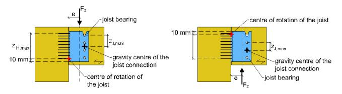
Figure B.1. Joist bearings fastened with nails and dowels for loading DOWN and UP
