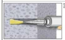
Starting from the bottom or back of the cleaned anchor hole, fill the hole up to approximately two-thirds with adhesive. Slowly withdraw the static mixing nozzle as the hole fills to avoid creating air pockets. If the bottom or back of the anchor hole is not reached, an appropriate extension nozzle must be used. Observe the gel-/ working times given in Table B5.
