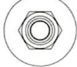
Configuration with internal thread and hexagon drive e.g. W-BS 6x55 TYP I M8/10
