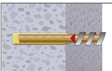
8. Insert the anchor rod while turning slightly up to the embedment mark.
