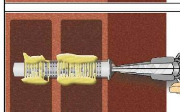
7. Starting from the bottom or back fill the sleeve with adhesive. For embedment depth equal to or larger than 130 mm an extension nozzle shall be used. For quantity of mortar attend cartridges label installation instructions. For push through installation the sleeve within the fixture must also be fully filled with mortar. Observe the gel-/ working times given in Table B4 + B5.
