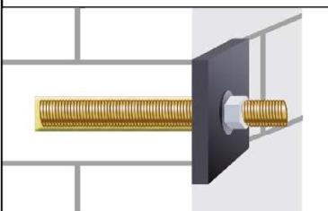
10. After full curing, the fixture can be installed with up to the max. installation torque (See parameters of brick Annex C4 to Annex C48) by using a calibrated torque wrench.
