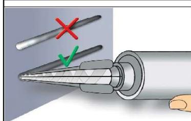
3. Initial adhesive is not suitable for fixing the anchor. Prior to dispensing into the anchor hole, squeeze out separately a minimum of three full strokes, for foil tube cartridges six full strokes and discard non-uniformly mixed adhesive components until the mortar shows a consistent grey colour.
