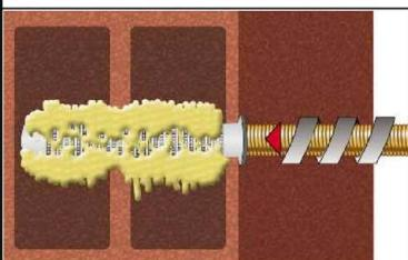
8. Push the threaded rod into the anchor hole while turning slightly to ensure positive distribution of the adhesive until the embedment depth is reached. The anchor shall be free of dirt, grease, oil or other foreign material.
