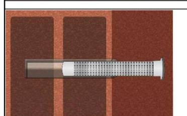
6. Insert the perforated sleeve flush with the surface of the masonry or plaster. Only use sleeves that have the right length. Never cut the sleeve. For installation through insulation the sleeve SH 16x130/330 shall be cutted at the top end according to the insulation thickness.
