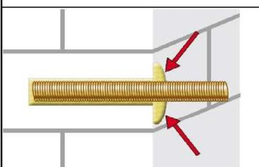
8. Be sure that the annular gap is fully filled with mortar. For push through installation the hole in the fixture must also be fully filled with mortar. If no excess mortar is visible at the top of the hole, the application has to be renewed.
