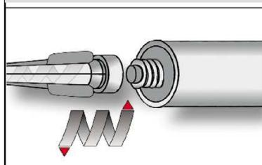
1. Remove the cap and attach the supplied static-mixing nozzle to the cartridge and load the cartridge into the correct dispensing tool. In case of a foil tube cartridge, cut off the clip before use. For every working interruption longer than the recommended working time (Table B4 and B5) as well as for new cartridges, a new static-mixer shall be used.
