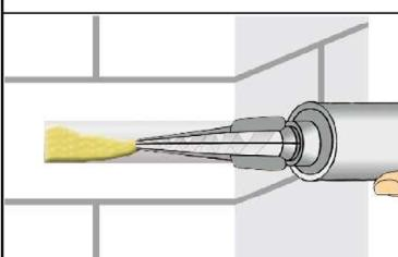
6. Starting from the bottom or back of the cleaned anchor hole, fill the hole up to approximately two-thirds with adhesive. Slowly withdraw the static mixing nozzle as the hole fills to avoid creating air pockets. If the bottom or back of the anchor hole is not reached, an appropriate extension nozzle must be used. Observe the gel-/ working times given in Table B4 + B5.
