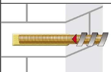
7. Push the threaded rod into the anchor hole while turning slightly to ensure positive distribution of the adhesive until the embedment depth is reached. The anchor shall be free of dirt, grease, oil or other foreign material.
