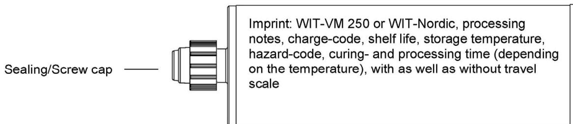
235 ml, 345 ml up to 360 ml and 825 ml Cartridge (Type: "side-by-side")
