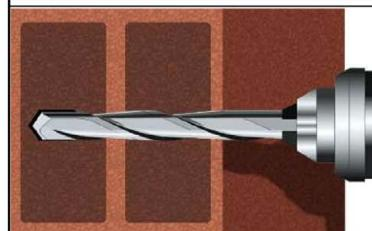
4. Holes to be drilled perpendicular to the surface of the base material by using a hard-metal tipped hammer drill bit. Drill a hole, with drill method according to Annex C4 – C48, into the base material, with nominal drill hole diameter and bore hole depth according to the size and embedment depth required by the selected anchor.
