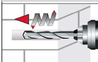
4. Holes to be drilled perpendicular to the surface of the base material by using a hard-metal tipped hammer drill bit. Drill a hole, with drill method according to Annex C4 – C48, into the base material, with nominal drill hole diameter and bore hole depth according to the size and embedment depth required by the selected anchor.
